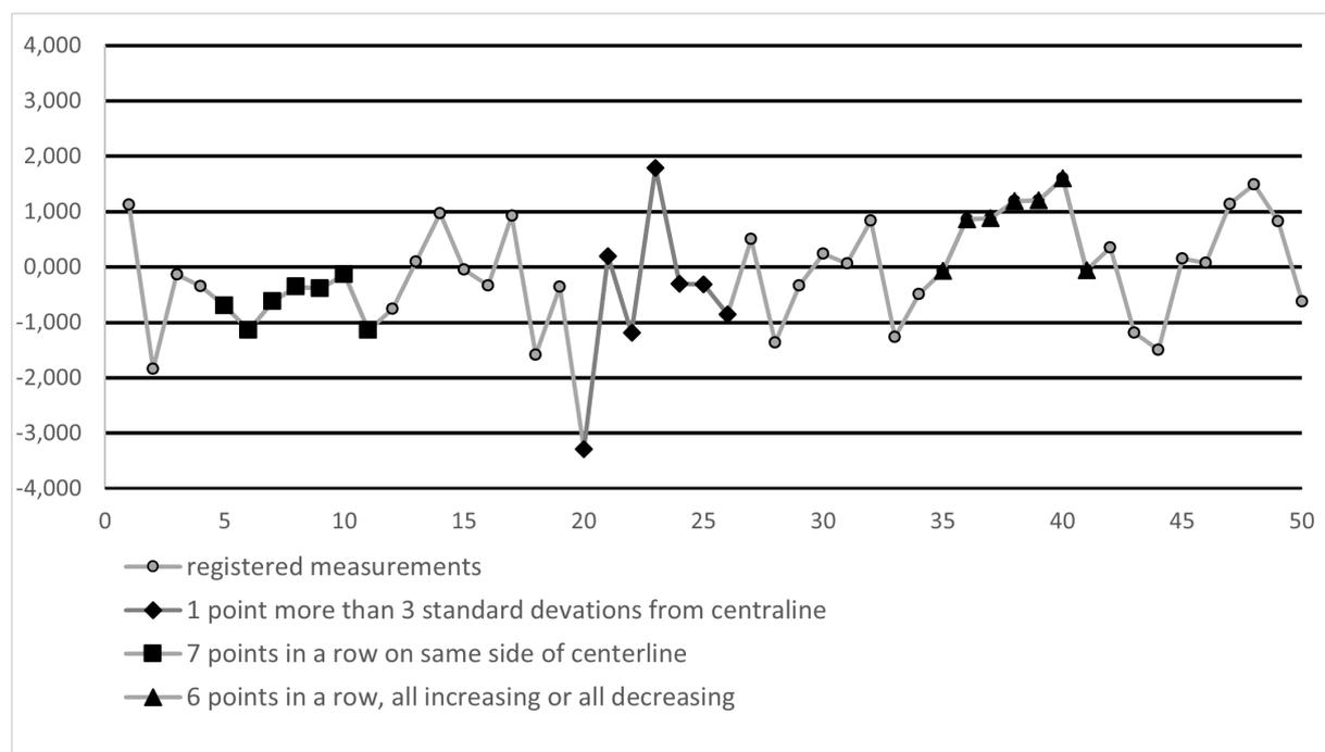
Fig. 4. Shewhart control chart for initial 50 samples
