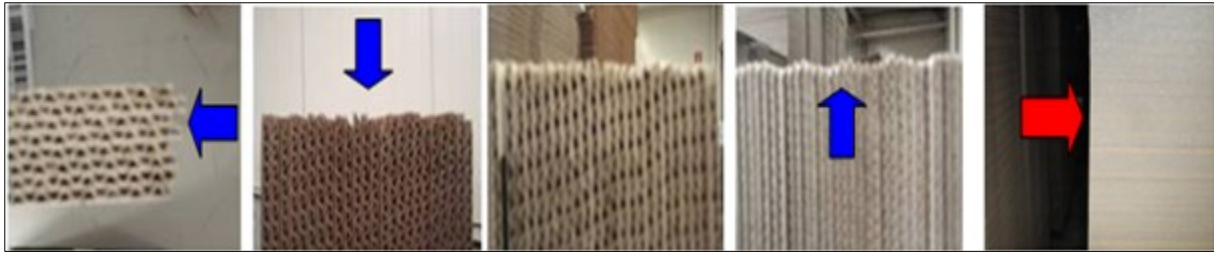
Fig. 2. Examples of cardboard cutting errors, the last photo is a cut in the norm
