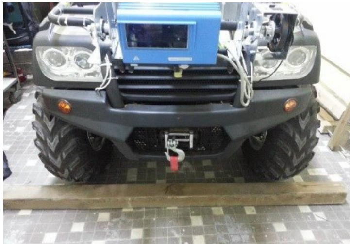
Fig. 2. Laser scanner and a wooden beam used as an obstacle during the tests
