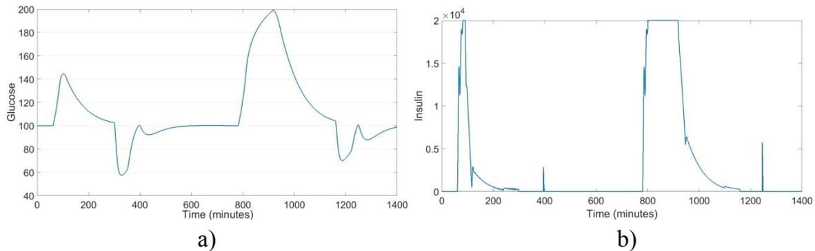
Fig. 6. Simulation results for a rule-based PID controller with constant parameters, meal and physical effort setup as in the Fig. 4, with a physical exercise and its prediction: (a) blood glucose; (b) insulin input
