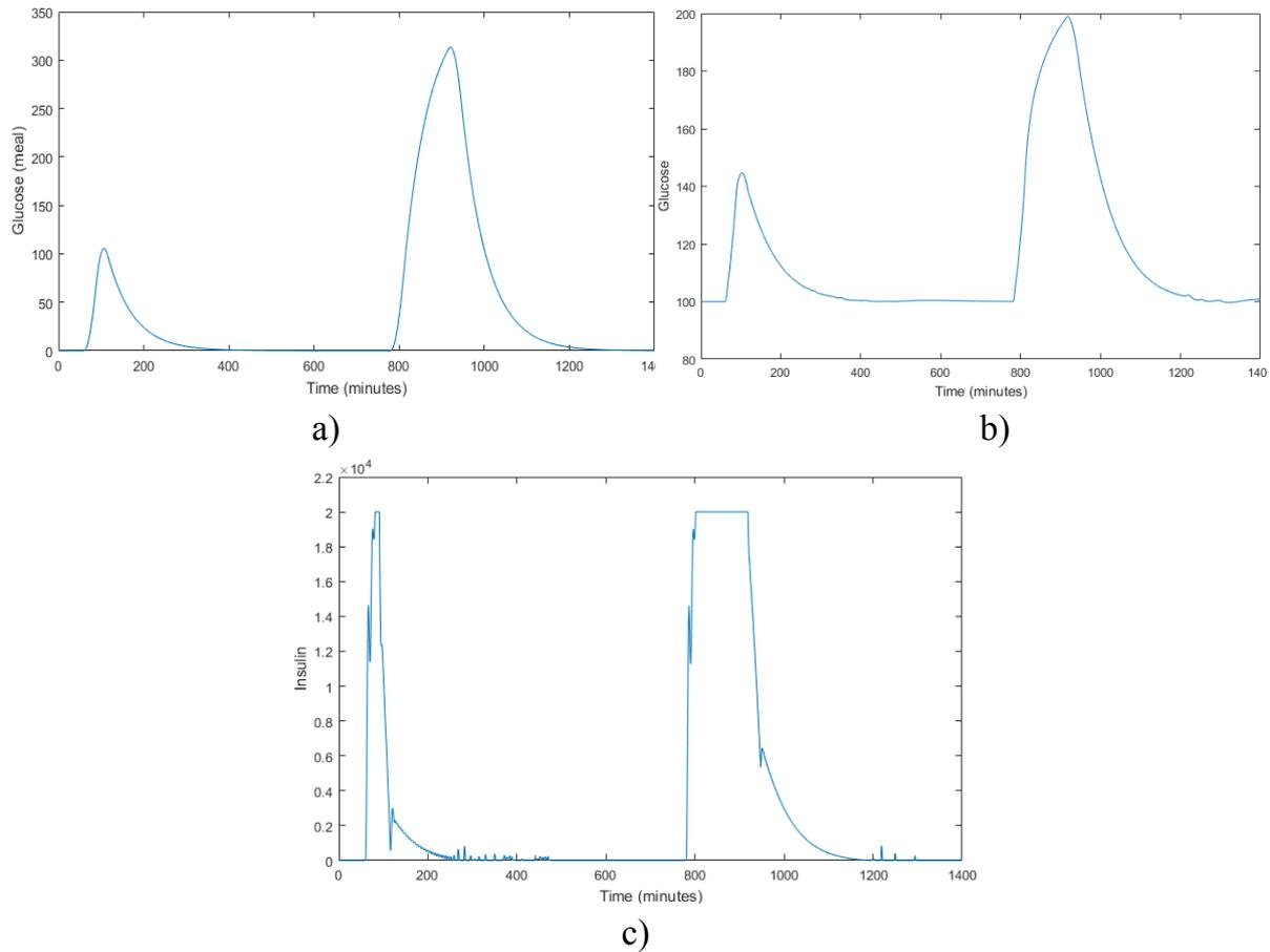
Fig. 3. Simulation results for a standard PID controller, without physical exercise: (a) glucose from the meals; (b) blood glucose; (c) insulin input
