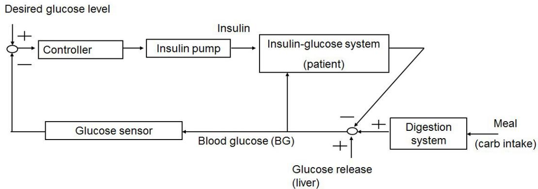
Fig. 1. A simplified block diagram of the control system
