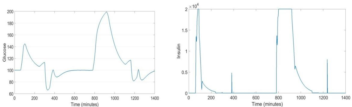
Fig. 7. Simulation results for a rule-based PID controller with a variable gain, meal and physical effort setup as in the Fig. 4, with a physical exercise and its prediction: (a) blood glucose; (b) insulin input
