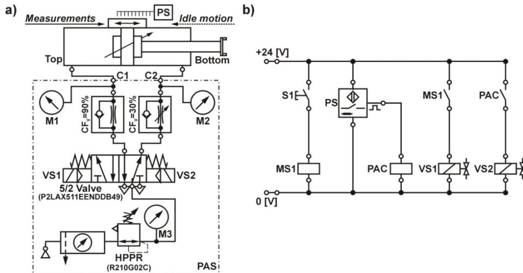
Fig. 4. Schematic functional diagram of the configuration: a) of the pneumatic drive, b) of electric connections to control the actuator
