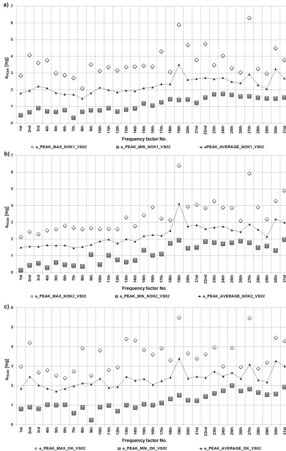
Fig. 7. Comparison of average values of acceleration from two independent measurement series in the defined frequency ranges measured by the sensor VS02 for the dampers: a) with defects (the first measurement series), b) with defects (the second measurement series), c) fully functional (the summary result from the two measurement series)
