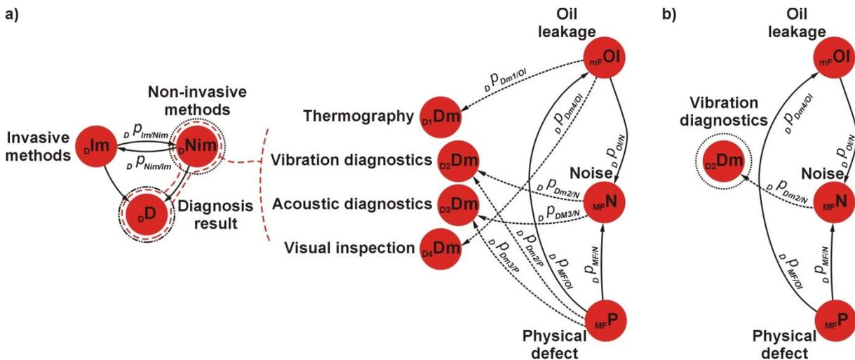
Fig. 2. A graph of available methods used for car damper diagnostics: a) complete graph, b) a graph after the reduction of paths
