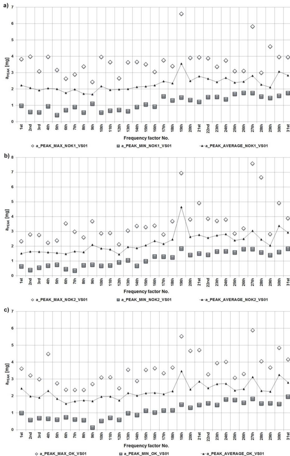
Fig. 6. Comparison of average values of acceleration from two independent measurement series in the defined frequency ranges measured by the sensor VS01 for the dampers: a) with defects (the first measurement series), b) with defects (the second measurement series), c) fully functional (the summary result from the two measurement series)
