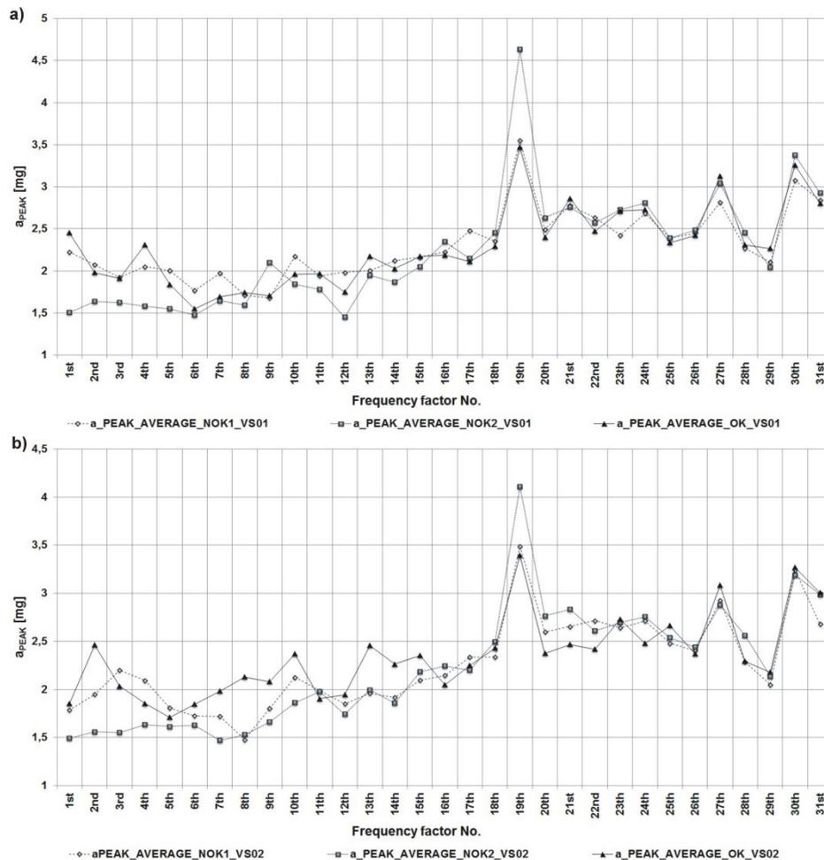
Fig. 8. Comparison of average acceleration values in the defined frequency ranges in two independent measurement series of the examined dampers with and without damages measured by the sensor: a) VS01, b) VS02
