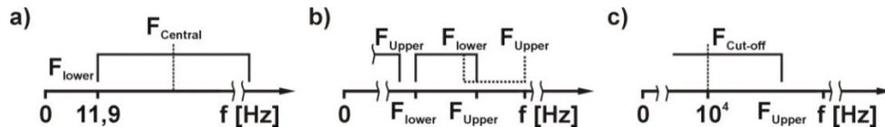
Fig. 5. Possible solutions of frequency range set for the measurements: a) at the beginning of the measurement range, b) within the range  $0 \div 10\text{kHz}$ , c) at the end of the measurement range
