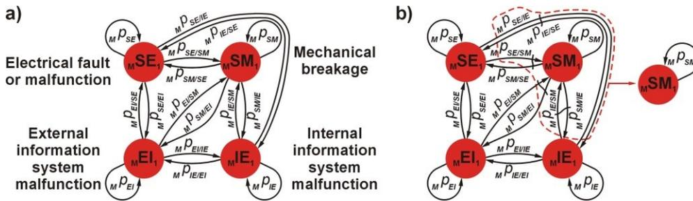
Fig. 1. General graph of the considered system: a) dependencies identified in relation to the development of defects, b) structures of the car damper; where:  $M_{SM}$  – mechanical structure,  $M_{SE}$  – electric structure,  $M_{IE}$  – internal stream monitoring information exchange,  $M_{EI}$  – external information exchange system,  $M_{Pa(i,j)b(i,j)}$  – element  $a_{(i,j)}$  on element  $b_{(i,j)}$  impact coefficient
